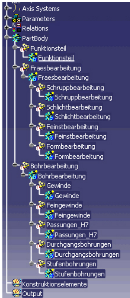
Figure 9 – Basic structure with corresponding body structure also valid for adapter
